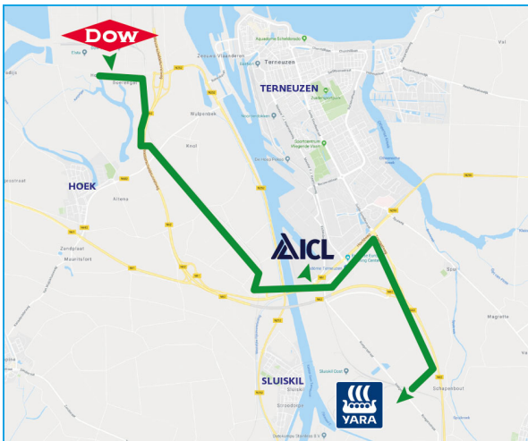
location of the hydrogen pipeline
